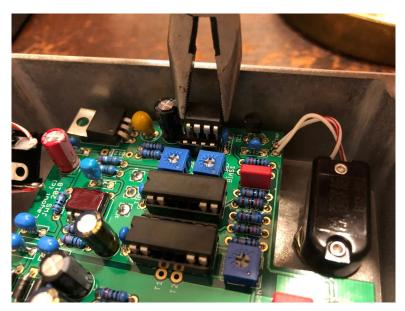
3. Very delicately, use an <u>IC extractor tool</u> or small needle-nose pliers to pull the old chip out of its socket. Don't pry too hard -- these are extremely fragile.
